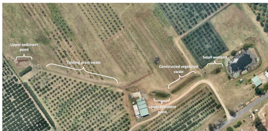
Figure 1: Site map showing the location of treatments systems at the Beenak site.
