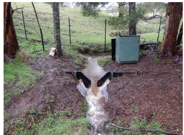
Figure 1. One of the flow and water quality monitoring stations in the Tarago catchment.
