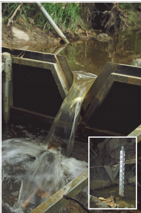
Above: One of four hydrological sampling points installed in the catchment, that record how much water flows down the creek. Inset: measuring staff used to measure water depth.
